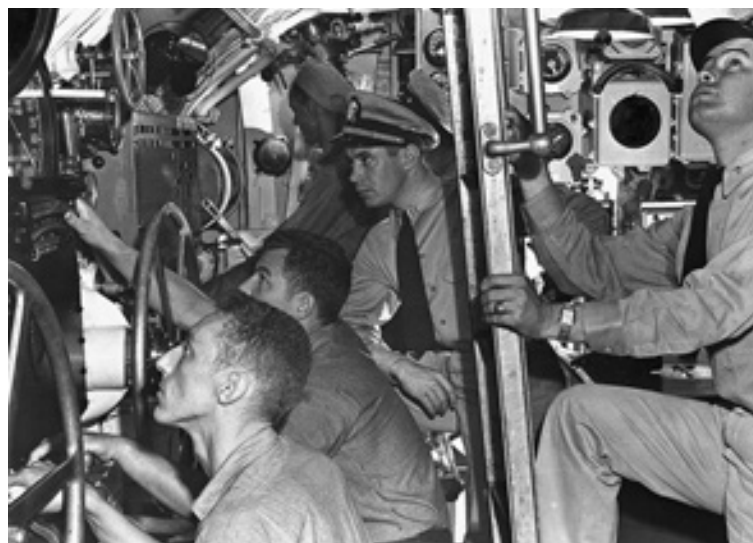
In old submarines, the "trimming" of a submarine to stay underwater was an intricate process, requiring the hand manipulation of countless valves by multiple sailors. In today's submarines, it's all done via computers at a central control station.
