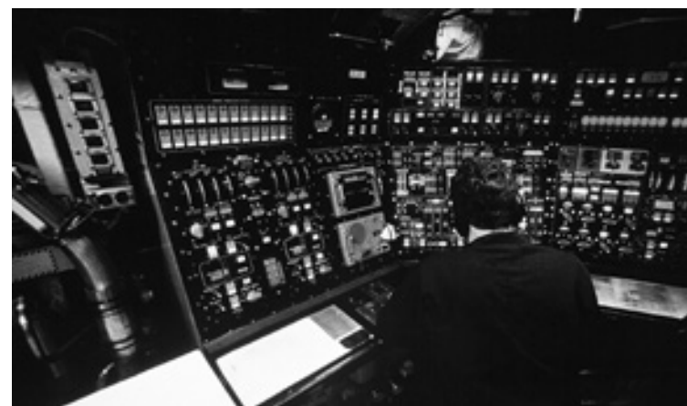
In old submarines, the "trimming" of a submarine to stay underwater was an intricate process, requiring the hand manipulation of countless valves by multiple sailors. In today's submarines, it's all done via computers at a central control station.
